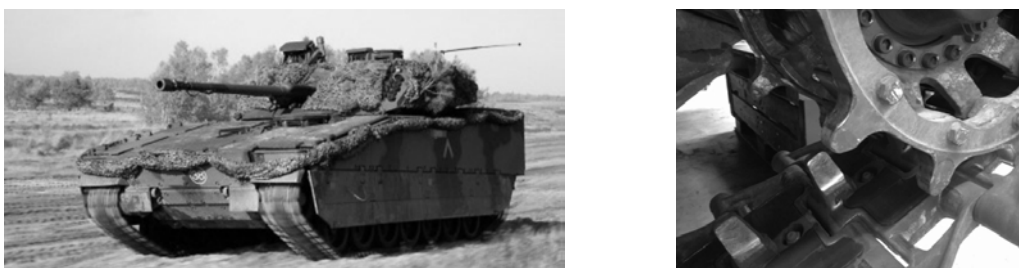
Figure 2: CV90 infantry vehicle, operating in a sandy environment and the sprocket wheel (right).
